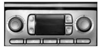
When your vehicle is first started and the climate control system is on, or if the climate control system has been turned on, the display will show the driver's temperature setting for five seconds. Then it will show the outside temperature.
